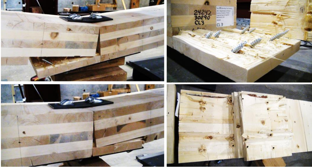
Figure 7 Failure mode of connected CLT panels under bending
